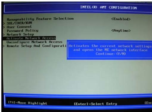
10. Your AMT client is set up successfully then exit MEBx
